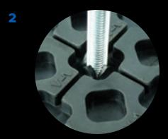
Install the anchor per anchor manufacturer's instructions, and push the pad over the installed anchor. The opening is designed to accommodate the size of the clamping hex nut required with concrete expansion anchors without interference.
