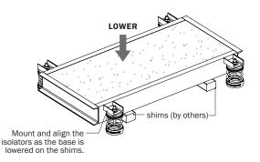
6. Place and anchor the equipment on base either with post-installed anchors or by using the optional cast-in-place bolts. See seismic calculations for embedment and edge distance requirements on anchors. Make sure that the orientation of the equipment is in agreement with the submittal drawing (motor end, pump end, etc.)
