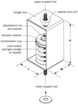
vertical uplift stopwasher (required for applications with seismic restraints)
